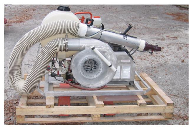
Truck-mounted electrostatic mist sprayer
