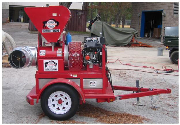
Truck/trailer mounted. Four Teejet 8502 nozzles in a cluster Flow rate up to 37.9 l/min
