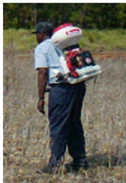
The hand portable sprayer provides the best way to apply Bti to many urban breeding sites. It is important to purchase a sprayer that is comfortable and easy to carry for several hours. Sprayers equipped with backpack or shoulder straps should be considered. The spray unit should hold two to four gallons and be equipped with a wand that has an adjustable nozzle.
